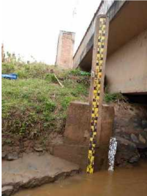
Figure 34: Limnometric scale on the Ruhwa River, Burundi (October 2020).
